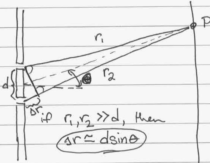
Pattern at P is superposition of 2 traveling waves
